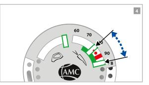
→ Watch the display on the Visiotherm further. Regulate temperature, as required:
